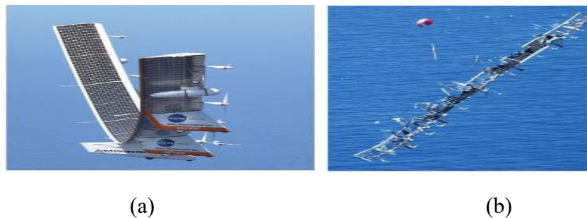
Figure 1.1 The crash of the NASA Helios aircraft (AR-31) (a) before crash and (b) after crash [12]
