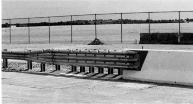
Figure 1.3: Energy absorber as road crash barrier [58].
